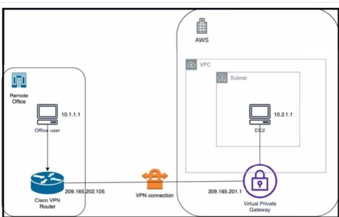
An engineer successfully brings up the site-to-site VPN tunnel between the remote office and the AWS virtual private gateway, and the site-to-site routing works correctly. However, the end-to-end ping between the office user PC and the AWS EC2 instance is not working.
