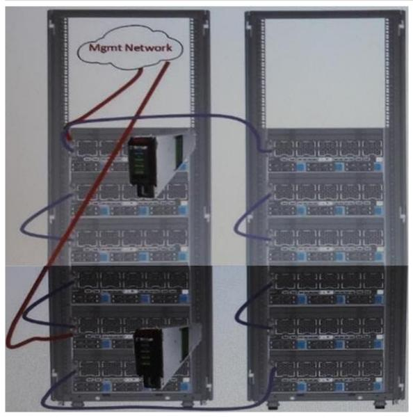
A customer with a 3-frame Synergy composable infrastructure has received a second rack to expand existing composable infrastructure resource pools. The integrator has cabled the management ring as shown. Which steps should the integrator take to increase availability of this configuration (Choose two.)
