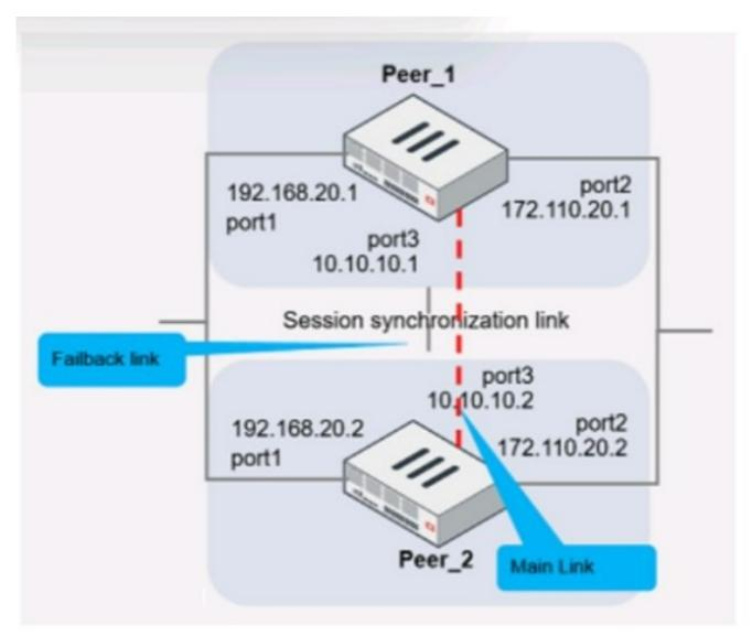
The main link directly connects the two FortiGate devices and is configured using the set session-syn-dev command.
